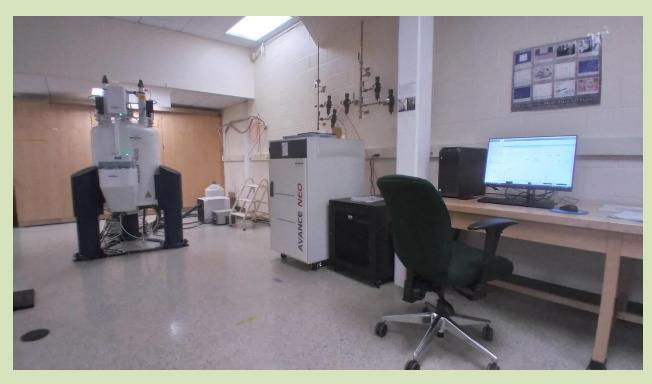
The newest addition to our spectrometer lineup is a Bruker Avance NEO 400 with solution and solid-state NMR capabilities.
